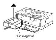
Insert the magazine (which has been taken out of the unit) firmly with the  $extbf{ iny}$  mark visible on the top side.
